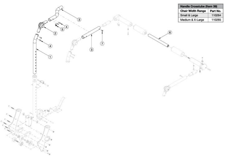
Callout #3: 10"-13" widths receive the curved tube and 14"-18" widths receive the straight shaped tube. When changing backrest types, check to see if new cables and tilt triggers are needed for both foot and hand tilts.
