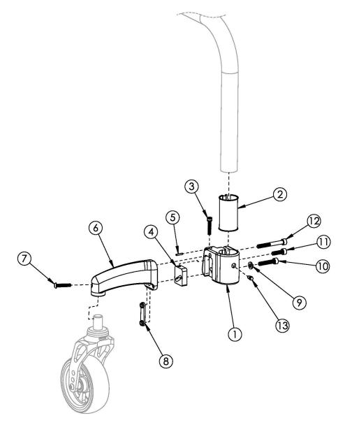
This design launched March 2016 If replacing a forward facing wing, quote opposite caster arm. The caster mount is an accent color option. When a chair is originally ordered, this part gets painted according to the accent color selection and not the frame color selection. Caster mount assembly does not include hardware please select appropriate hardware kit for full assembly.
