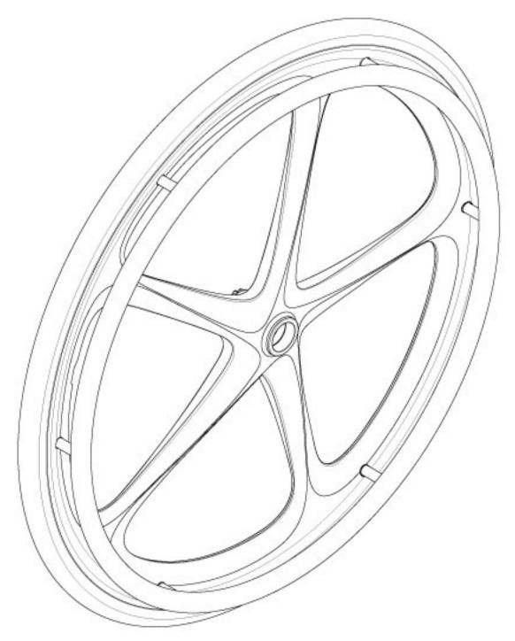
Not all components of the Wheel, Tire and Handrim kits will be listed. If changing wheel size and anti-tips are present, new anti-tips may be required. If changing wheel size or style, new axles, receivers, and/or axle plates may be needed.
