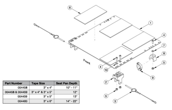
This is an Aluminum Seat Pan for Transit Use. Requires Seating System Cross Braces. The width and depth of the seat pan will measure approximately 0.5" shorter than the listed description.
