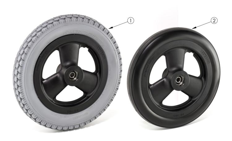
If changing wheel size and anti-tips are present, new anti-tips may be required. If changing wheel size or style, new axles may be needed.
