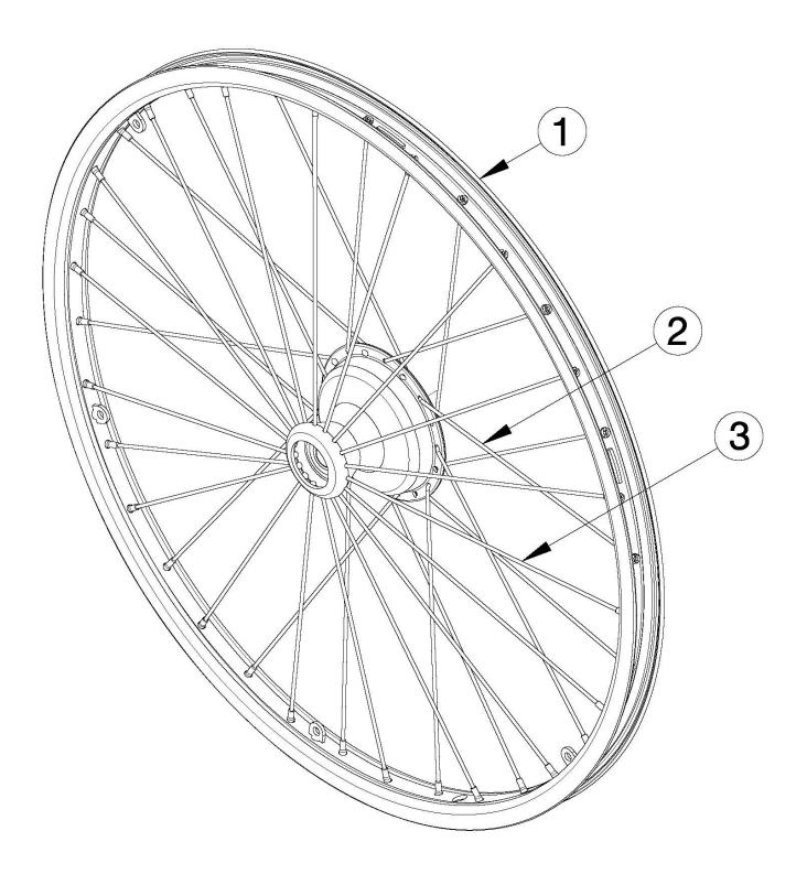
If changing wheel size and anti-tips are present, new anti-tips may be required. If changing wheel size or style, new axles and/or receivers may be needed. New wheel locks might be needed when changing wheel size or style.
