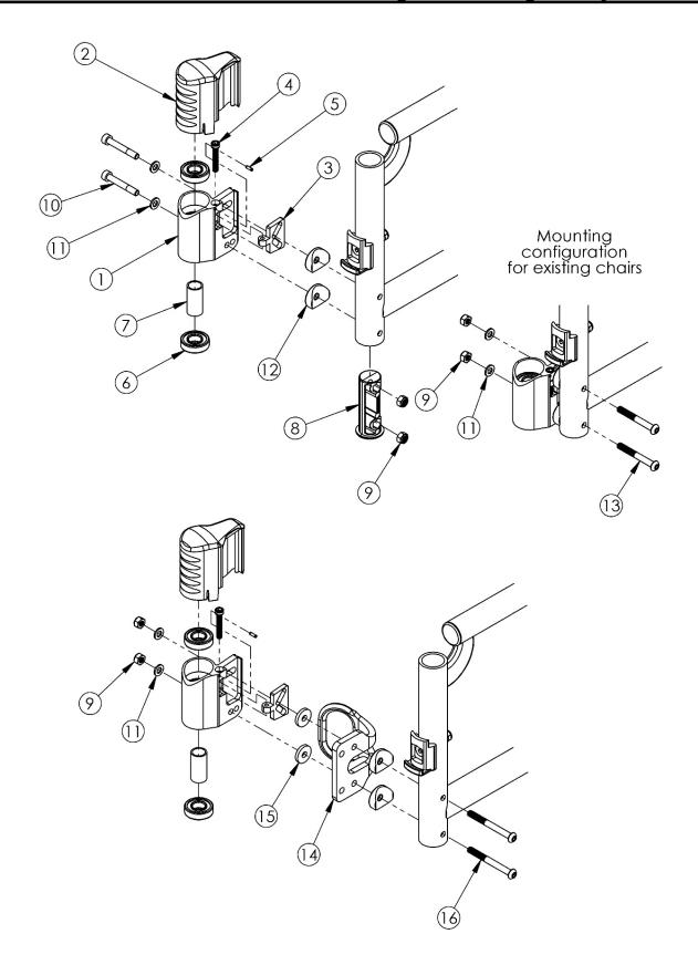
Please Note: The shown orientation of the caster housing above is in the "Forward" position. If only 1 side caster housing is needed, customer must confirm the orientation of the caster housing.
