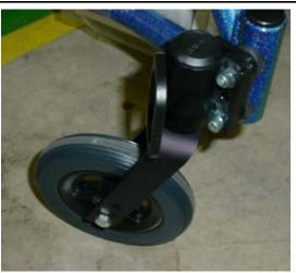
Figure 13: Final Setup with Caster Barrel Trailing
