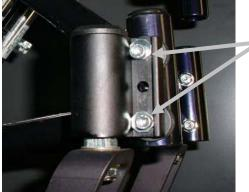
Remember Orientation of Eccentric Washer to help in the reinstallation in later steps.
