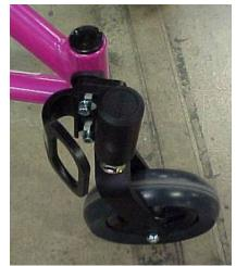
Figure 12: Final Setup with Caster Barrel Leading
