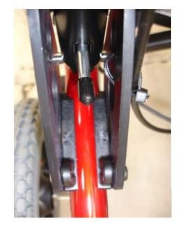
Figure 1a: New Saddles and Vertical Supports
