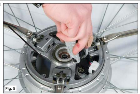
5) Gently feed the sensor through the opening in the wheel assembly. (Fig 6)
