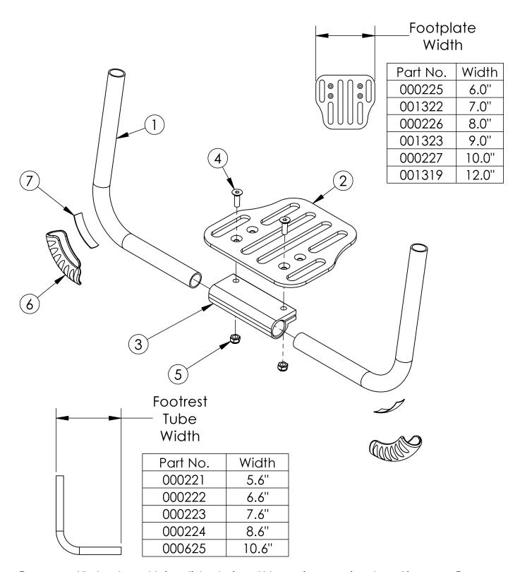
Footrest assemblies based on straight frame If changing from a high mount footrest to a frame inserted footrest on a Rogue or Tsunami, please see the appropriate Rigid Frame page for necessary hardware. On Tsunami, if footrest is installed prior to December 2012, new attaching hardware is required.
