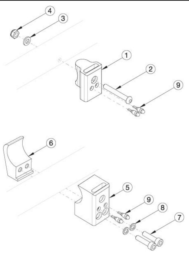
If retrofitting side guards, clamp on receiver is required
