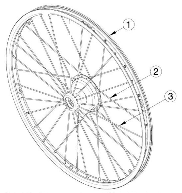
If changing wheel size and anti-tips are present, new anti-tips may be required. If changing wheel size or style, new axles may be needed. Please note tab mounted handrims must be installed prior to the tire being installed.
