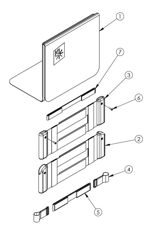
Open Back Wings (3a - 3l) are used when integrated push handles are present. Closed Back Wings (2a - 2l) are used when back posts without push handles are present. Tension Straps (7a and 7b) are used with the combination of Fold Down Push Handle and Padded Velcro Adjustable Back Upholstery and are based on chair width.
