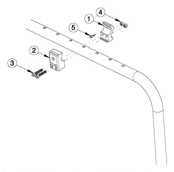
Color anodized versions of this receiver may not contain the two counterbored holes at the bottom of the receiver
