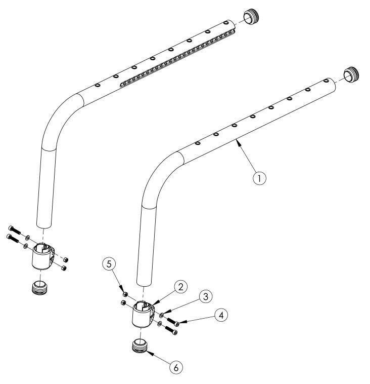
This Clik Side Frame is discontinued and was used on serial numbers prior to CLK005270. Item numbers 2-5 are only needed when footrest is not high mounted.
