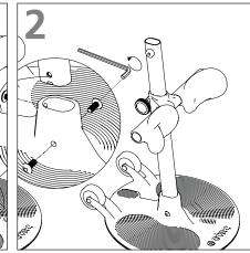
Place the base plate on an Insert all three screws into holes in the base plate. Use allen key to screw in bolts. Tighten bolts firmly.
