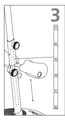
The knee support height can be read from the scale on the pole. The number above the leg support bracket referes to the correct height.
