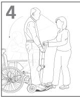
Step on footrest, brace your weight and ask the user to sit down. Maintain eye contact with the user during the entire transfer prococess.
