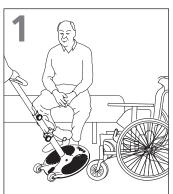
Position the new seat (chair, wheelchair, toilet or bed) in an 90 degree angle with the existing seat.
