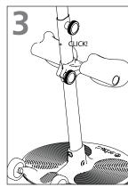
There will be a clicking sound when it is correctly mounted. Turn and tighten the knob.
