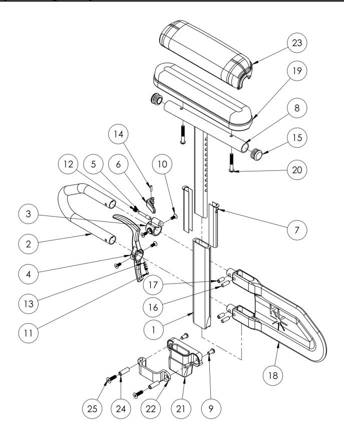
Short assemblies are used with 14-17 Seat Depths. Long assemblies are used with 18"-19" Seat Depths
