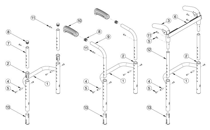
Utilize this page when retrofitting to the Rigid Locking Fold Down Back on a Rogue 10, Rogue ALX or Ethos. If chair shipped after 7/3/2025 and Rigidizer Mounted Stroller Handles are present, please refer to quote the appropriate Stroller Handle Page for the Rigidizer.
