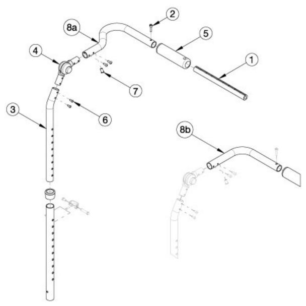
Has your width changed? Will the push handle (#8) accommodate your new width? If no, please select the appropriate upper back tube assemblies. If chair was invoiced prior to 12/18/23, an upper back tube assembly is required. If chair was invoiced after to 12/18/23, upper back tube assembly can now be purchased individually
