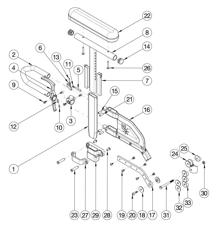
Receiver and Hardware update effective 11/25/24 Short Side Shield used with 14"-17" Seat Depths. Long Side Shield used with 18"-20" Seat Depths If retrofitting, Receivers are needed. If retrofitting to Height Adjustable Flip Back T-Arms and One Arm Drive is present, a new drive shaft may be required. In addition to a new drive shaft, order the corresponding hardware kit: 109438 for Blade Style One Arm Drive, 503433 for Hex Style One Arm Drive or 112898 for Quick Release Style One Arm Drive
