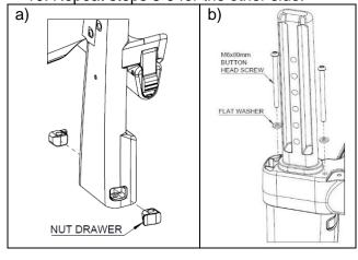
11. Set the seat and back assembly onto the base frame. Ensure all four legs of the seat are aligned with the four slotted holes in the
