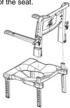
Insert the two M6x80mm button head screws with flat washers into holes on the underside of the seat. Tighten the screws into the nut drawers to secure the backrest to seat.
