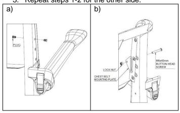
Attach the chest belt by looping through the slot on the chest belt mounting plates.
