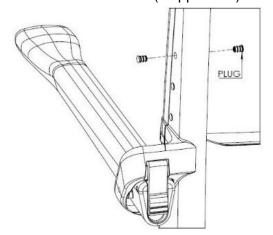
2. Insert the M6x40mm button head screw into the backrest and chest belt mounting plate. **Hand tighten** the lock nut.
