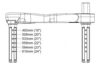
13. Insert the height adjust clips through all 4 legs of the base and seat.
