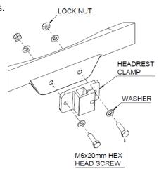
2. Insert the headrest assembly into the headrest clamp, adjust to the appropriate height and tighten the tri-lobe.
