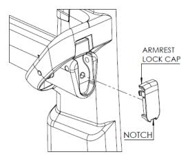
3. Using a hammer, tap in the knurled pin through the arm and armrest lock, smooth side first. *Flip the arms up for better access to armrest.*
