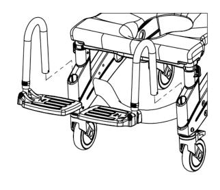
15. Ensure the notch on the hanger tubes sits securely on the pin in the footrest receiver hole.
