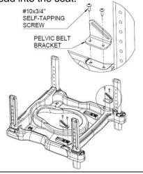
Attach pelvic strap by looping through slot on pelvic belt brackets.
