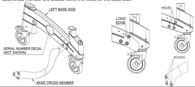
2. Secure the base side and base cross member with three M6x40mm button head screws with flat washers and hinged caps.
