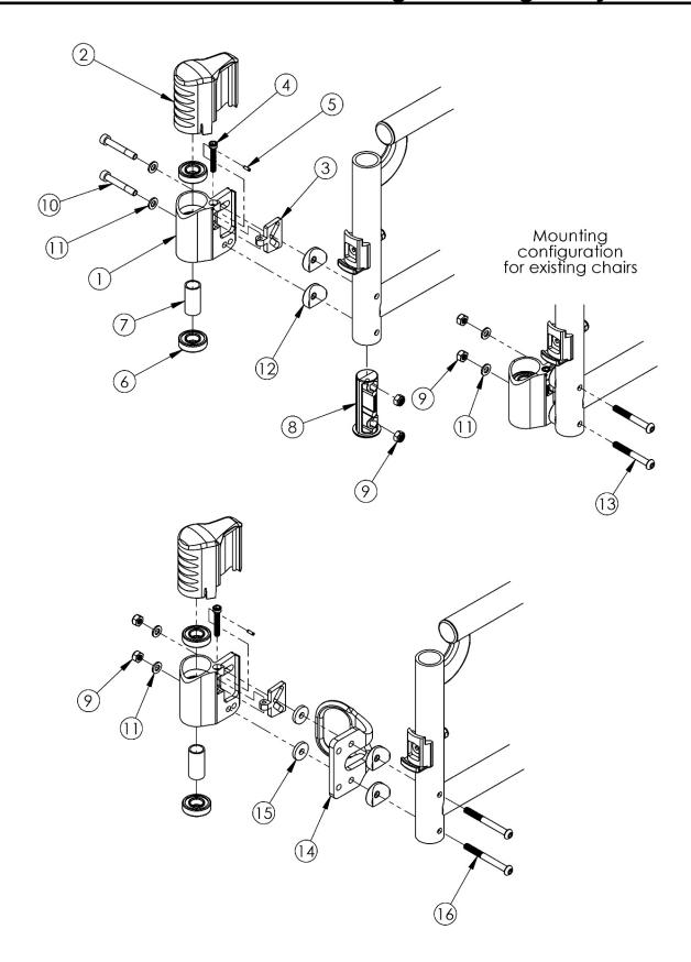
Please Note: The shown orientation of the caster housing above is in the "Forward" position. If only 1 side caster housing is needed, customer must confirm the orientation of the caster housing.
