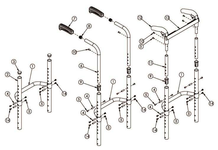
If chair was ordered with Rigid Locking Fold Down Back, please see Rigid Fixed Height Back Post with Adjustable Height Rigidizer Bar page. Effective on Rogue starting with serial number RG0016612. If retrofitting to this backrest on Rogue, a new backrest mount and hardware may be required. Tension Straps (#13) are based on seat width and used in combination with back upholstery.
