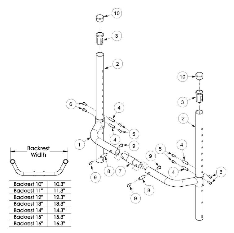
Adjustable Height Rigidizer Bar based on seat width
