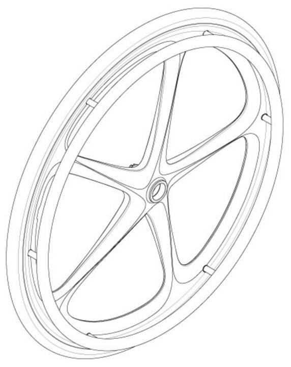
Not all components of the Wheel, Tire and Handrim kits will be listed. These kits cannot be used if Drum Brake is present. If changing wheel size and anti-tips are present, new anti-tips may be required. If changing wheel size or style, new axles and/or receivers may be needed. For the Catalyst 4, new axle plates may be needed. See Rogue2 Axles page for axle and receiver utilization.
