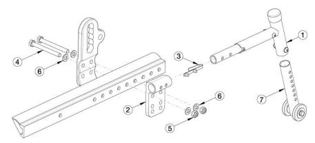
Anti-Tip assemblies are based on rear wheel size. Anti-Tip Receivers are installed on Focus chairs. Receivers are not needed when retrofitting anti-tips to a chair unless removing the Vent Tray and replacing the Vent Tray Anti-tips with the Focus CR Rear Anti-tips.
