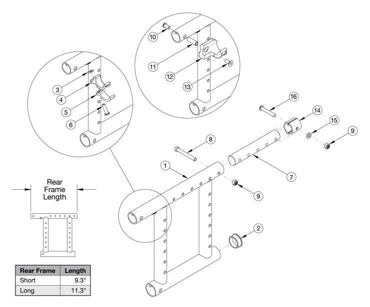
Use short frame for 14-17" Seat Depths. Use long frame for 18-20" Seat Depths If changing to a new seat depth, new Height Adjustable T-Arms may be required
