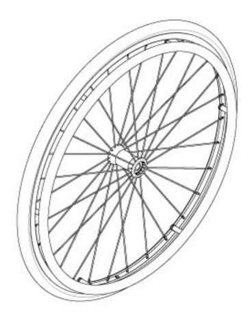
Not all components of the Wheel, Tire and Handrim kits will be listed. If changing wheel size and anti-tips are present, new anti-tips may be required. If changing wheel size or style, new axles and/or axle plates may be needed. These kits cannot be used if Drum Brake is present.
