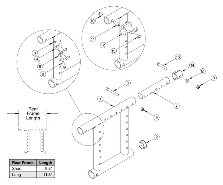
Use short frame for 14-17" Seat Depths. Use long frame for 18-20" Seat Depths If changing to a new seat depth, new Height Adjustable T-Arms may be required If retrofitting Rear Frame, Depth Adjustable Extension with Hardware needed
