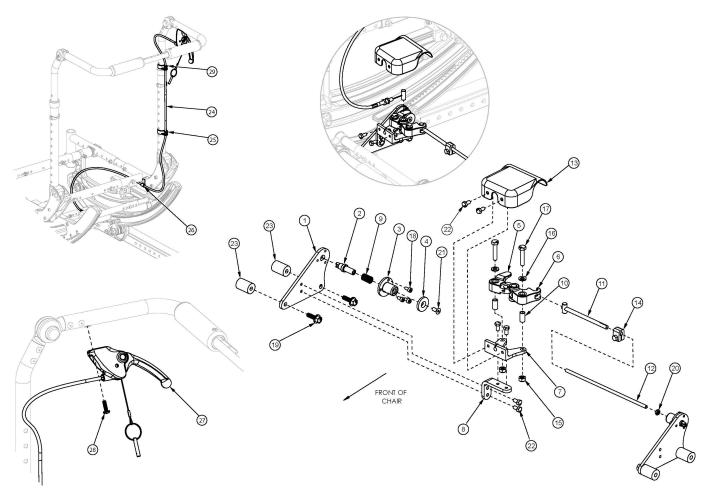
This design effective starting with serial numbers FCR0026599 and FCHD002333. If serial number is prior to FCR0026599 and FCHD002333 new upper back cane assemblies are required in addition to the hand tilt mechanism.
