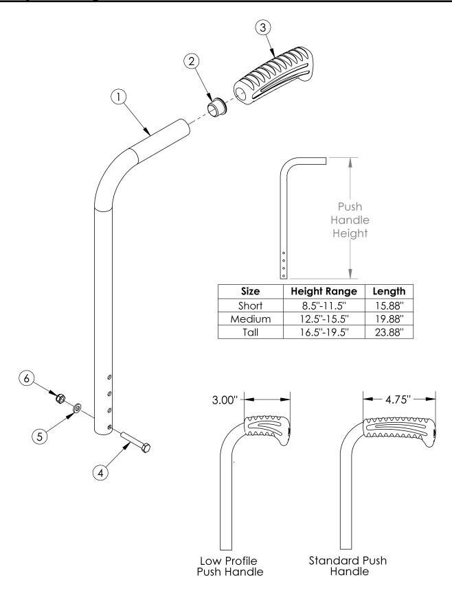
Low Profile Push Handles are not available with Heavy Duty Option or Drum Brake If changing from another style backrest and the Drum Brake is present, a new Drum Brake Cable Kit may be required If Anti-Rollback is present, see Back Tubes for Anti-Rollback System
