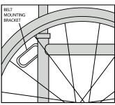
**Figure 8.** Wheelchair Belt Restraint Anchor
