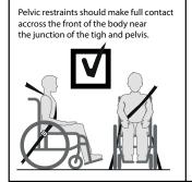
Belt restraints must not be held away from the body by wheelchair components such as armrests or wheels.
