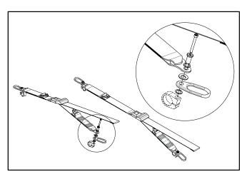
Figure 9. Wheelchair-anchored Belt Restraint
