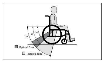
Figure 5. Recommended Pelvic Belt Placement Angles
