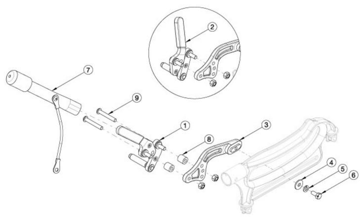
Please note: If a "Dual Drum Brake" is present, items 8 and 9 are required. The Arc Wheel Lock Mount is the same across all styles of Wheel Locks and is not needed if changing Wheel Lock styles.
