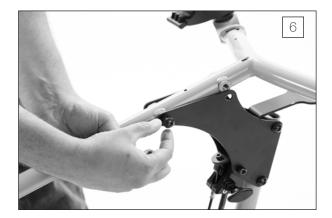
7. Once all 4 bolts have been started, tighten all 4 bolts securely. Place unit onto its wheels.
