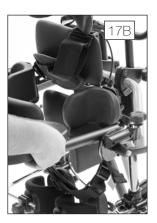
18. Remove head support and place the stem into the clamp as shown. Tighten securely.
