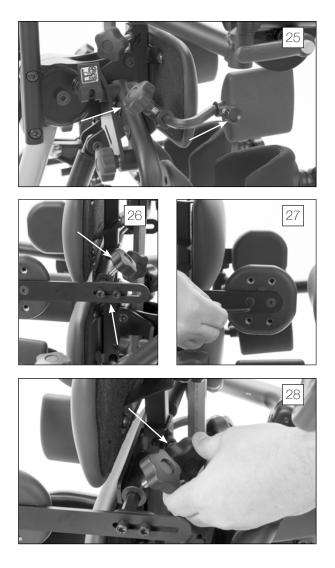
Calf Pad with Knee Strap 29. To adjust the calf pad with knee strap, loosen knobs on each side. Position fore/aft and up/down to the desired setting. Tighten securely.
