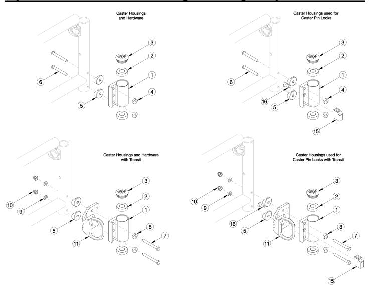
Please Note: The shown orientation of the caster housing above is in the "Forward" position.
