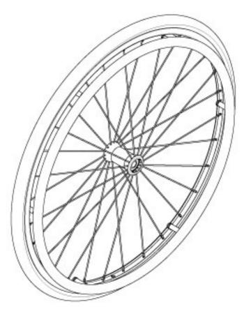
Not all components of the Wheel, Tire and Handrim kits will be listed. These kits cannot be used if Drum Brake is present. If changing wheel size and anti-tips are present, new anti-tips may be required. If changing wheel size or style, new axles may be needed. For the Catalyst 4, new axle plates may be needed.
