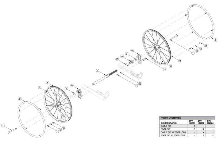
Effective 5/13/2022, all One Arm Drives will be shipped with a close mounted handrim on the non-drive wheel. Not available with Attendant Foot Lock. If changing wheel size and the Attendant Foot Lock is present, a new linkage may be required; reference the corresponding Focus CR Attendant Foot Lock page.
