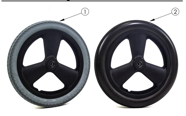
If changing wheel size and anti-tips are present, new anti-tips may be required. If changing wheel size or style, new axles may be needed. if changing wheel size and Attendant Foot Lock, spacer 112503 is required which can be found on the CR45 Axle Plate page
