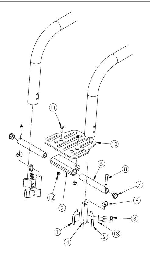
Footrest assemblies based on straight frame Used on serial numbers prior to TS010953, TSHD003973, TSTR004735, RGXP008523, RGX0020821, and RG0018443
