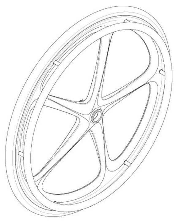
Not all components of the Wheel, Tire and Handrim kits will be listed. These kits cannot be used if Drum Brake is present. If changing wheel size and anti-tips are present, new anti-tips may be required. If changing wheel size or style, new axles and/or receivers may be needed. New wheel locks might be needed when changing wheel size or style.
