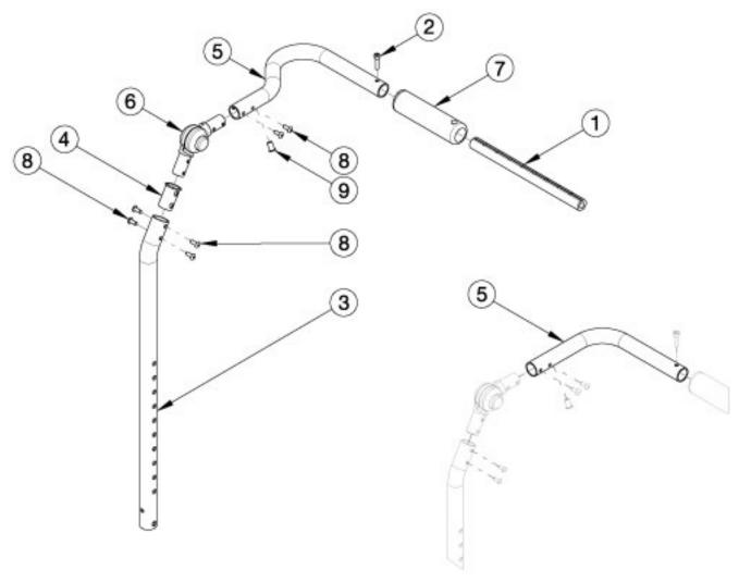
Has your width changed? Will the push handle (#5) accommodate your new width? If no, please select the appropriate back assembly. Callout #5: 10"-13" widths receive the curved handle and 14"-18" widths receive the "L" shaped handle. If chair width is 14"-18" wide and has a serial number of FLP010784 through FLP011079, see the Discontinued Flip Fixed Height with Adjustable Handle Backrest page.
