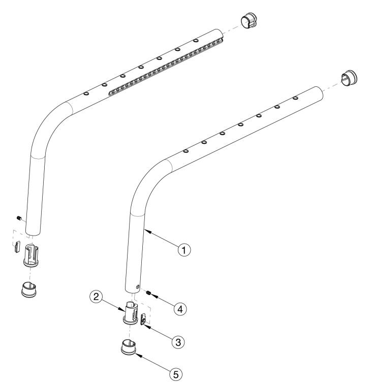
This design effective starting with serial numbers CLK005270. Drilled Clik Side Frames effective April 13, 2018. Replacement side frames may be quoted, but must be ordered through Customer Service. Serial number required upon order. Item numbers 2-4 are only needed when footrest is not high mounted and these parts are included with replacement side frames if footrest is not high mounted. If quoting a Left Frame for Australia or New Zealand, 122921 is required when transit is not present.
