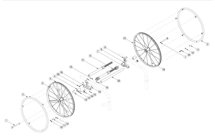
Most One Arm Drive kits do not include rear tires. If retrofitting to add the One Arm Drive, new rear towers are required in addition to the complete One Arm Drive system and camber tube kit. Effective 5/13/2022, all One Arm Drives will be shipped with a close mounted handrim on the non-drive wheel. Used on chairs invoiced prior to 3/12/25
