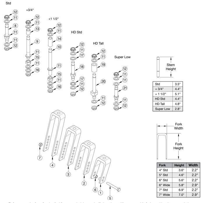
Reference order form for detailed front seat height matrix. If changing to 2" casters, wide forks and hardware needed.
