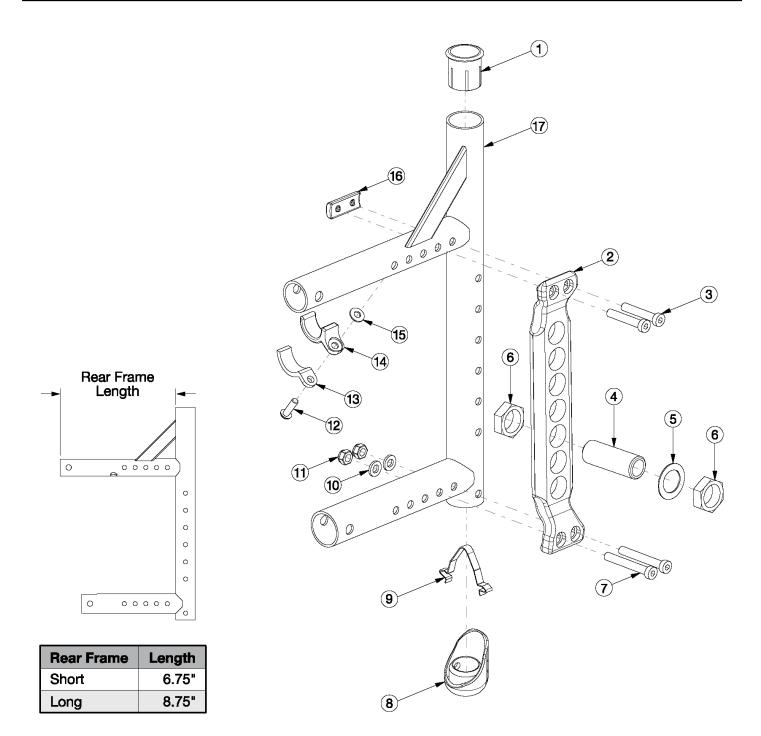
Retrofitting to this axle plate and rear frame requires 300lb or 350lb Weight CapacityUse short frame for 14-17" Seat Depths and long frame for 18-20" Seat Depths
