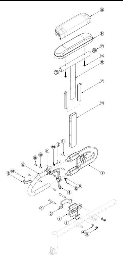
If retrofitting, Receivers are needed. Callout #3: Spacer is needed when the receiver sits on the seat growth tube. Callout #6: Depending upon the placement of the receiver will depend on the length of screw you'll need. More specific information is on the way! Please note there is a receiver screw and spacer kit that includes all potential screw sizes and spacer (you will need qty 2 for a pair).
