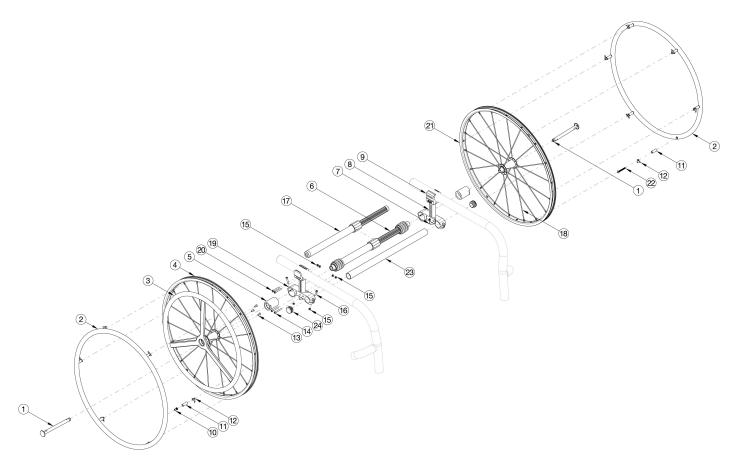
Most One Arm Drive kits do not include rear tires. If 24" Pneumatic w/ Airless Insert tires are needed, please see kits that include those tires. If retrofitting to add the One Arm Drive, new rear towers are required in addition to the complete One Arm Drive system and camber tube kit. Effective 5/13/2022, all One Arm Drives will be shipped with a close mounted Aluminum Anodized Handrim on the non-drive wheel.
