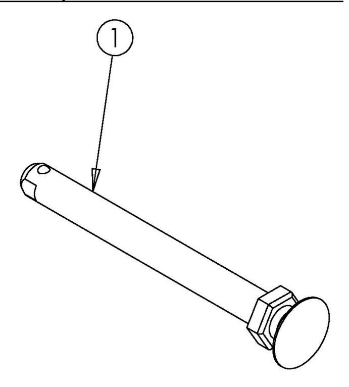
Utilizes Axle Sleeve 100756 (Reference parts manual page "Flip for Leckey Rear Frame").
