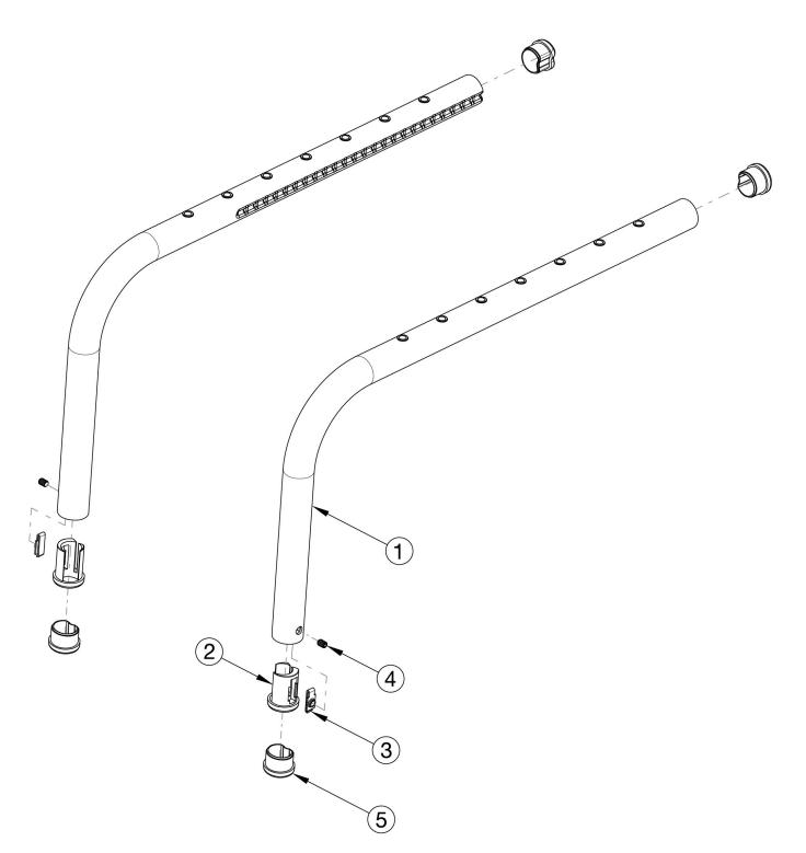
This design effective starting with serial numbers CLK005270. Drilled Clik Side Frames effective April 13, 2018. Replacement side frames may be quoted, but must be ordered through Customer Service. Serial number required upon order. Item numbers 2-4 are only needed when footrest is not high mounted and these parts are included with replacement side frames if footrest is not high mounted.
