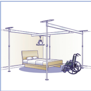
The 4 post Easytrack operates like a traditional x-y system covering all 4 corners of a room. The 4 post system is not telescopic
